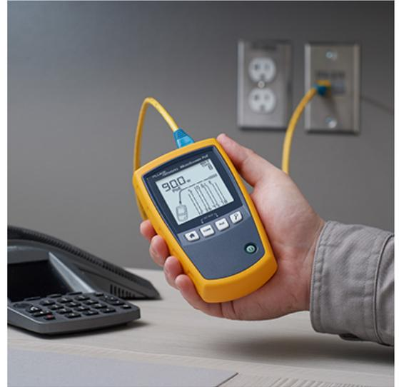
*Figure 5. The MicroScanner PoE can detect the power offered by the PSE plus the network's speed, and features a suite of cable testing features.*
