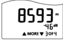
The end of the link. The length of the link (without the launch fiber) is 8463 m.
