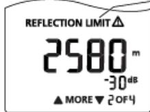
A bad splice on the fiber at 2450 m caused a reflectance incident that is larger than -45 dB (the default limit).
