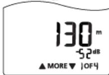
The reflectance of the first connection is -52 dB. The length of the launch fiber is 130 m.
