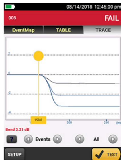
Bend as seen on an OTDR trace
