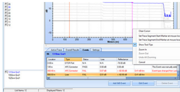
Setting span event parameters using LinkWare PC
